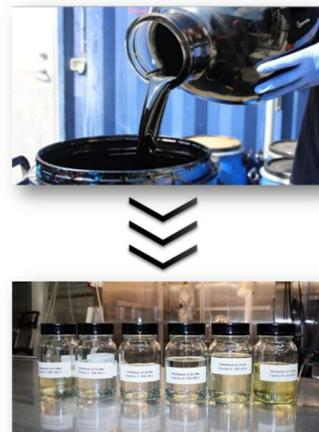
**Figure 5:** Pictures of crude oil and the clear fractions of the upgraded product.
